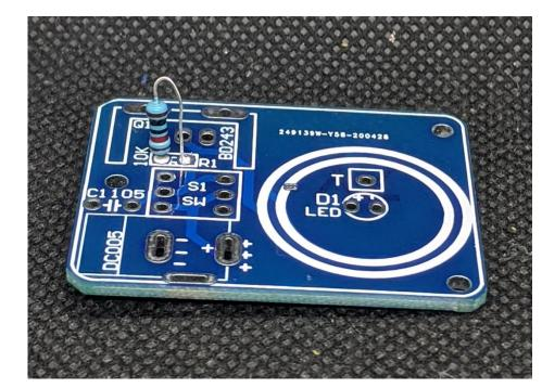
**2.** Start by soldering the 10K resistor as shown. Inserting this way allows the resistor to fit onto the PCB
